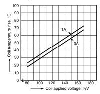
5-(2). Coil temperature rise (200 mW Standard type) Tested sample: HY1Z-12V, 5 pcs. Ambient temperature: 23°C 74°F
